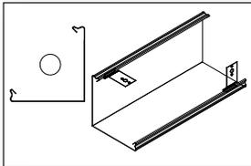
Choose the U-Shield profile when three sides of your pipe or mechanical need to be covered.
